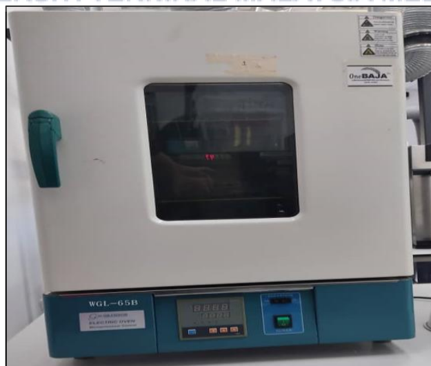
Figure 3. 5 GAINSON WGL-65B electric drying oven
