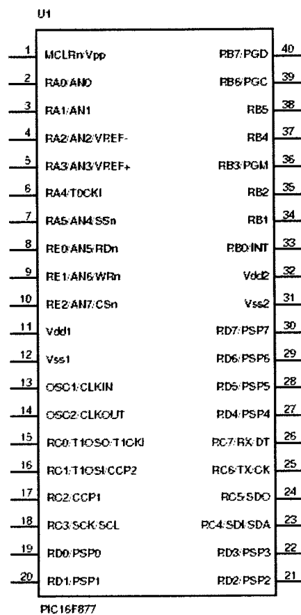
Figure 2.5: The assignation of 16F877A pins.
