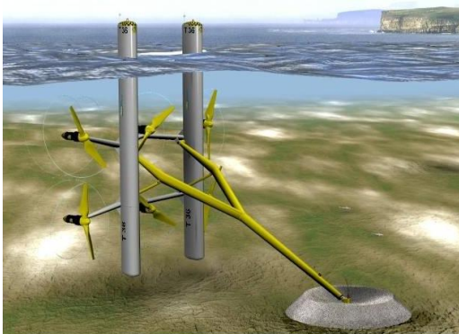
Figure 2.5: Tidal Stream Technology use at river [17].
