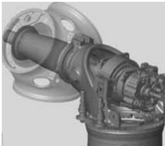
Figure 1-7: Part of the driveshaft connecting the rotor to the drivetrain, housed inside the nacelle. (Gardner, P)
