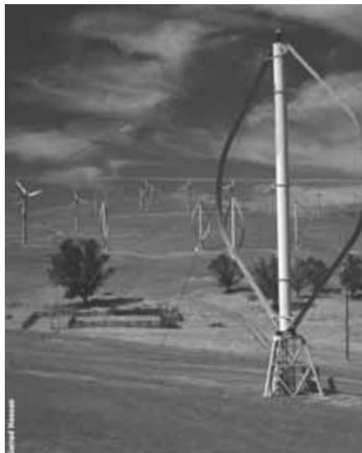
Figure 1-5: Darrieus-type VAWTs (Gardner, P)
