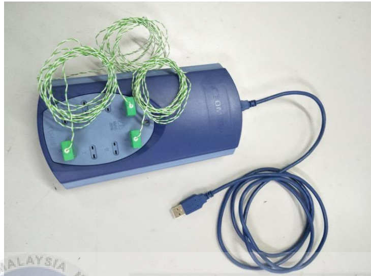
Figure 3.7: Data logger (USB TC-08) with K-type thermocouple
