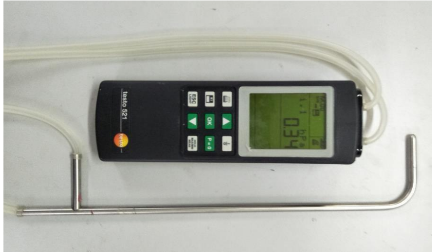
Figure 3.6: Pitot tube (Testo 0635 2145 L-Type) with digital manometer (Testo 521-1)
