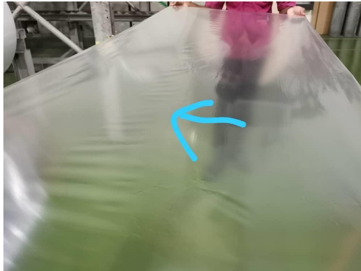
Figure 1.1: Baggy web defect on BOPP films.
