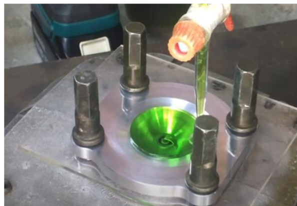
Figure 3.14 Cylinder head machining and volume measurement.
