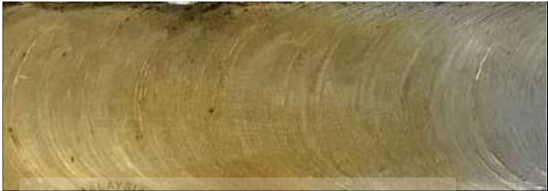
Figure 2.9 Surface Topography of UFSW
