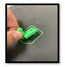
2. Clean up filament residues on the nozzle and bed.
