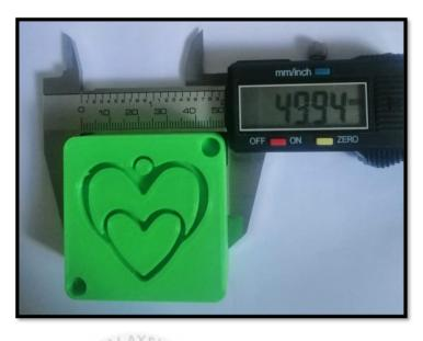
Figure 27 Dimensional Error on Lower Die
