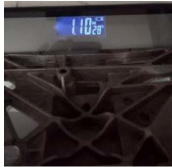
Figure 3.7 Weighing of Based Model Engine Mounting Bracket
