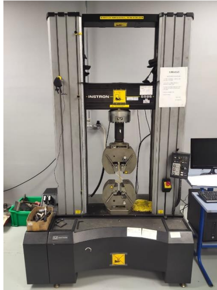
Figure 3.6 INSTRON FLOOR MOUNTED MATERIAL TESTING SYSTEM (2000kN) for tensile test
