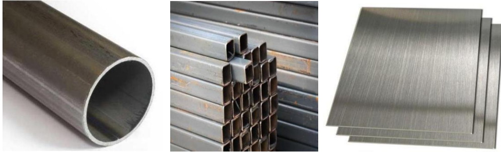
Figure 3.11 Circular Hollow, Square Hollow and Plate Steel.
