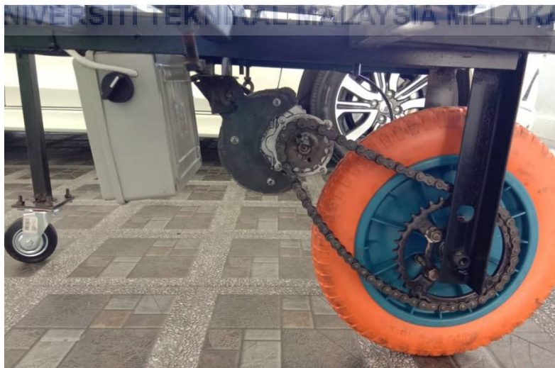
Figure 4.7 The Frame of the Motor Part attached with the Motorized Trolley
