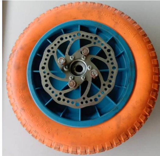
Figure 4.13 Non Pneumatic Tire with Disc Rotor
