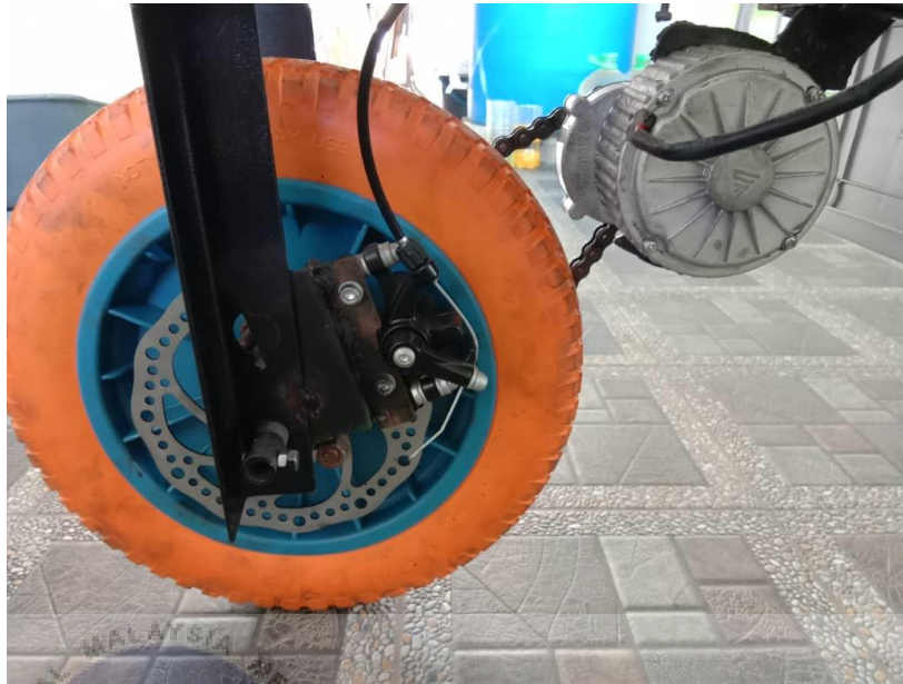
Figure 4.9 The Brake System of the Motorized Trolley
