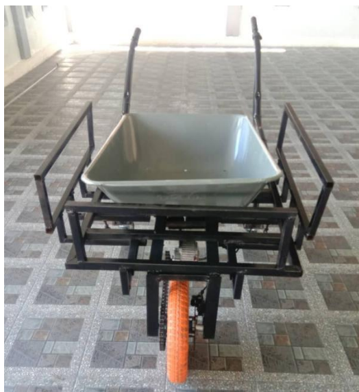
Figure 4.14 Motorized Trolley with the Steel Tray
