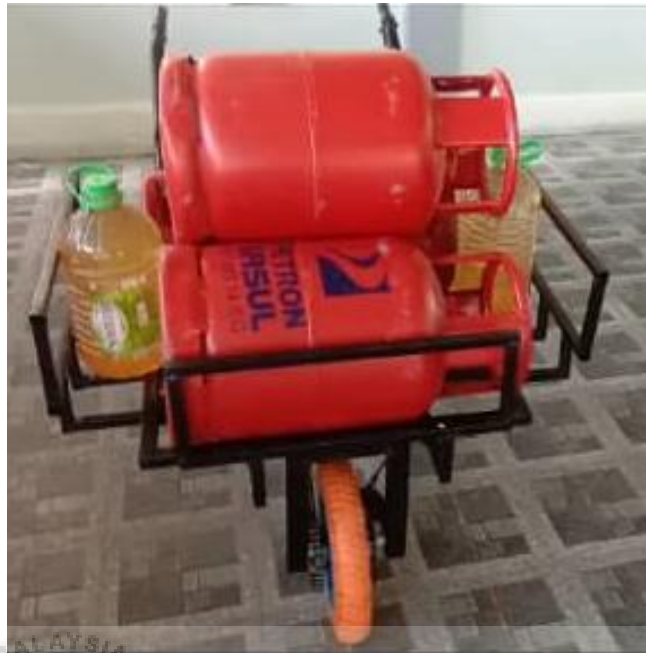
Figure 4.17 Motorized Trolley with the Maximum Loads of 100KG
