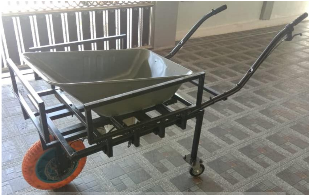
Figure 4.16 Motorized Trolley with an Extendable Frame
