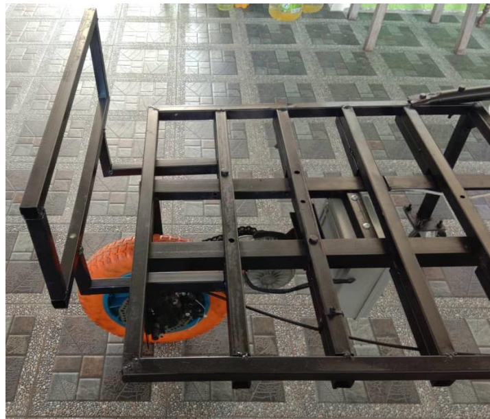
Figure 4.3 Front Extendable Frame on the Motorized Trolley
