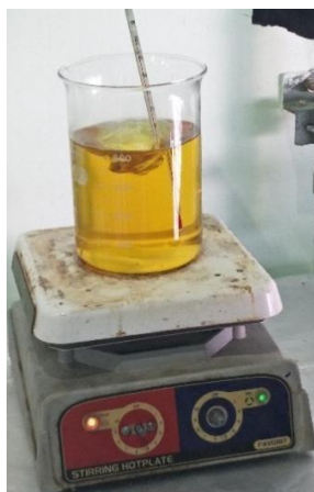
Figure 3.3.2 Heating biodiesel with stirring hotplate
