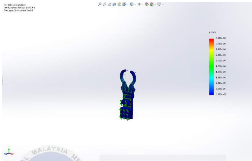
Figure 4.11: 8 Newton load for Normal Strain
