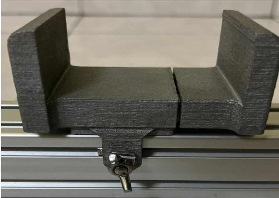
Figure 4.13 Butterfly head screw M5 used as a lock holder
