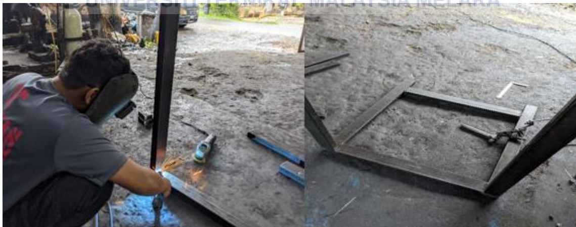
Figure 3.10 Frame welding process using MIG
