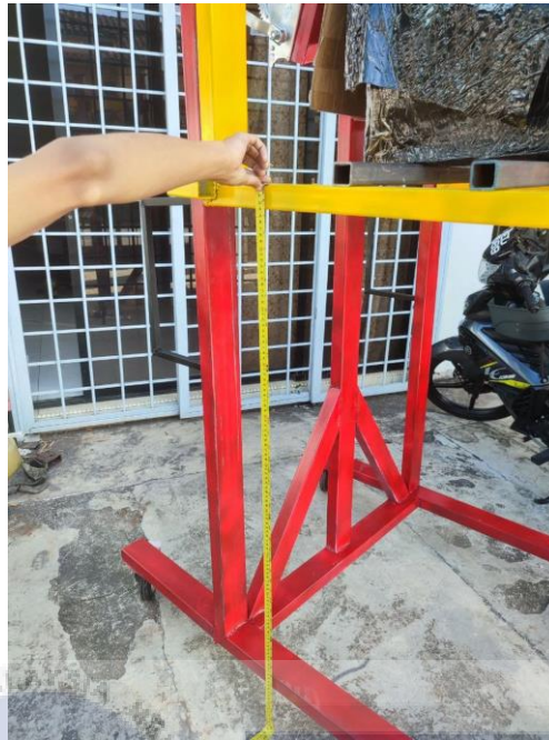
Figure 4.13 Fork maximum height
