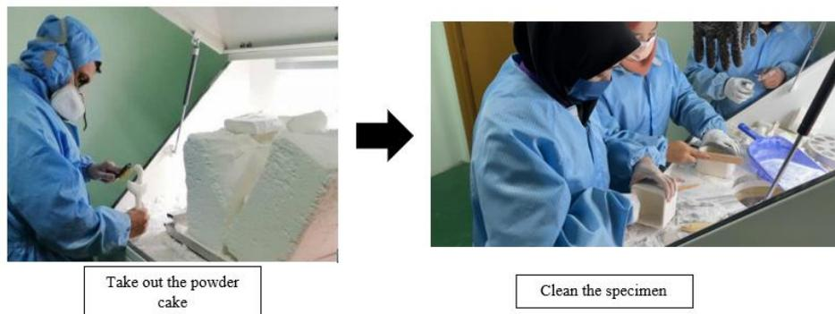
**Figure 3. 4** post-process 3D Printer
