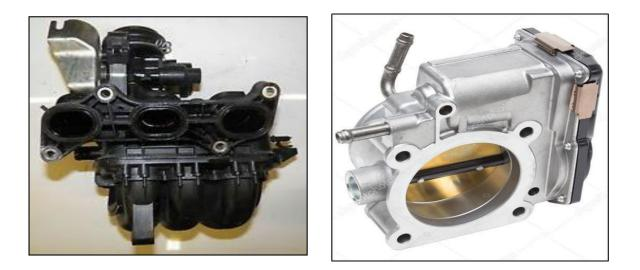
Figure 2.3: The intake manifold and throttle body play major role in air intake system [11]
