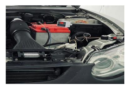
The digital temperature controller measuring air intake temperature
