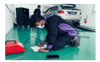
Measured and obtain the emission value manually from the EMS gas analyser
