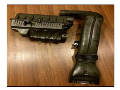
Figure 3.4: Satria Neo Air Filter 1.6L
