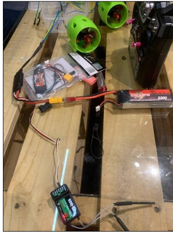
Figure 4.7 ESC calibration RC controller to RC receiver
