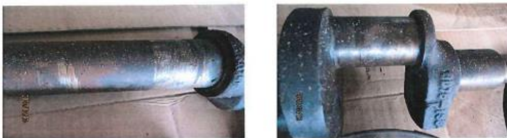
Figure 3-3 Both Picture shown Deep Scratch on Crankshaft compressor
