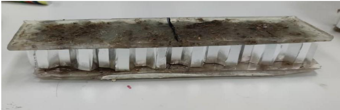
Figure 4.1 Sandwich honeycomb panel with oil palm fibre reinforced with resin polyester
