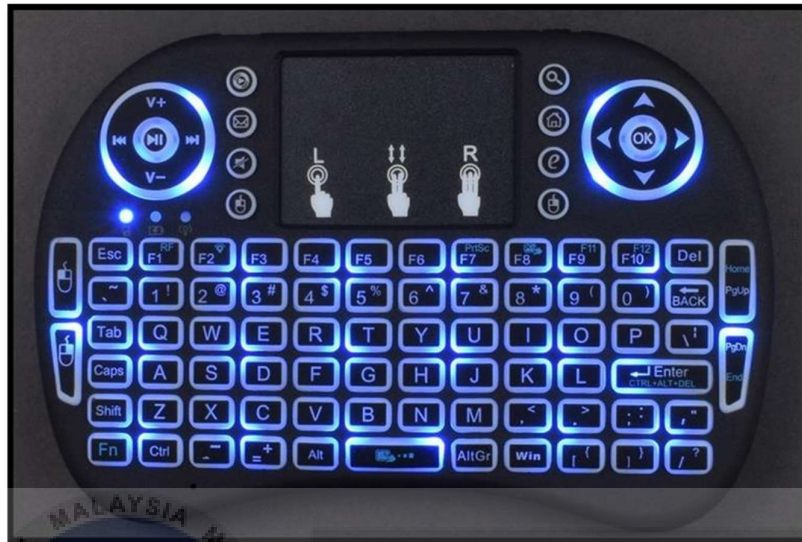
Figure 3.8: Wireless Keyboard with Lithium battery
