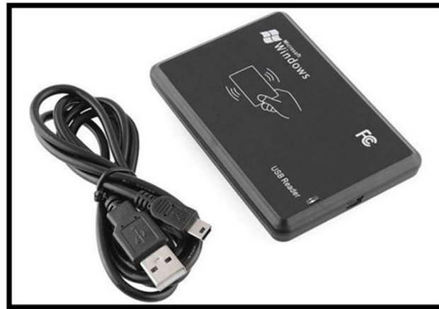
Figure 3.6:: USB RFID reader Smart ID Card Reader EM4001(125Khz)
