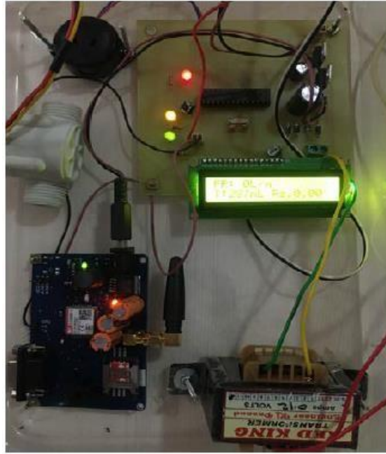
Figure 2.5: Circuit construction of Smart Water Meter
