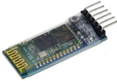
Figure 3.9: HC-05 Bluetooth module
