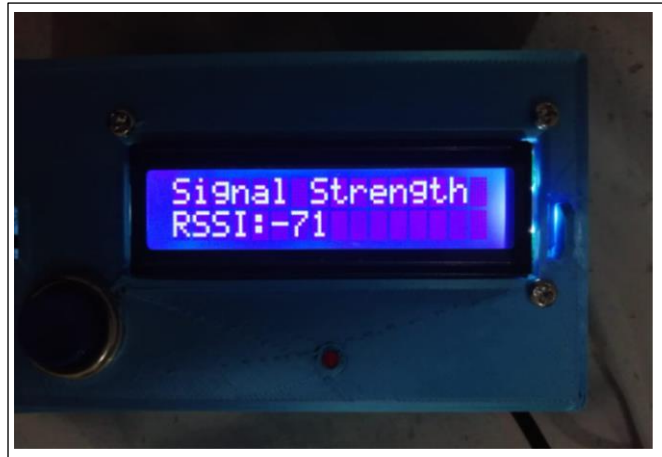
Figure 4.13: Signal Strength of the LoRa module
