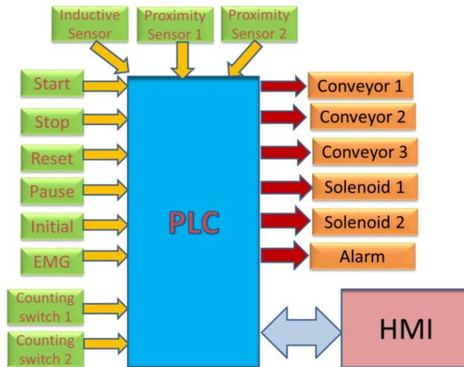
Figure 2.17 Block diagram of automation packaging system Pro-face remote HMI
