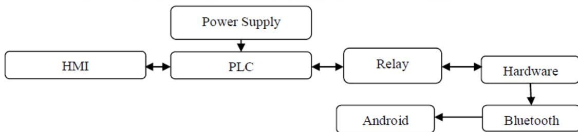
Figure 2.2 Block Diagram of Control and Monitor System
