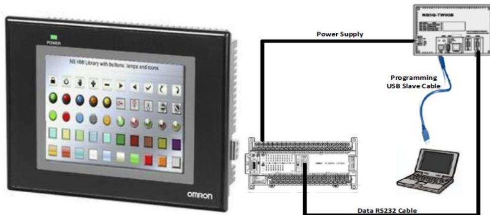
Figure 2.3 Hardware Connection of HMI Omron NB7W-TW00B
