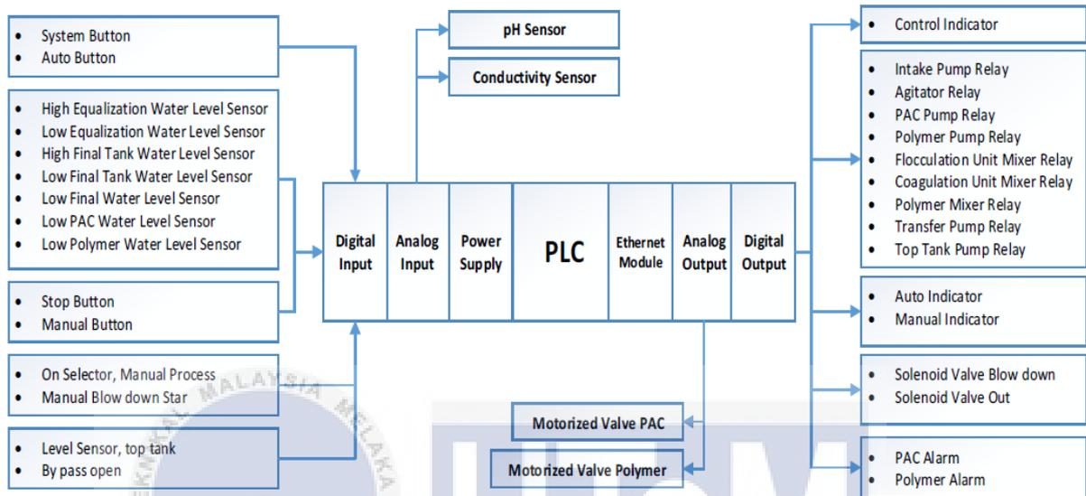
Figure 2.22 Input-Output Block Diagram of PLC
