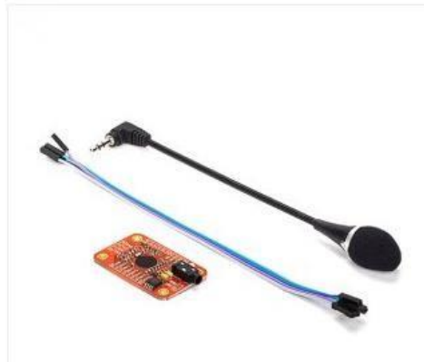
Figure 3.8 Components of the Voice module
