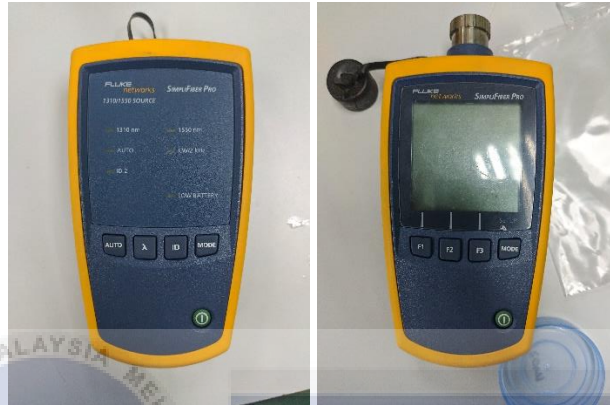
Figure 3.5 Optical Power Level and Optical Power Meter.
