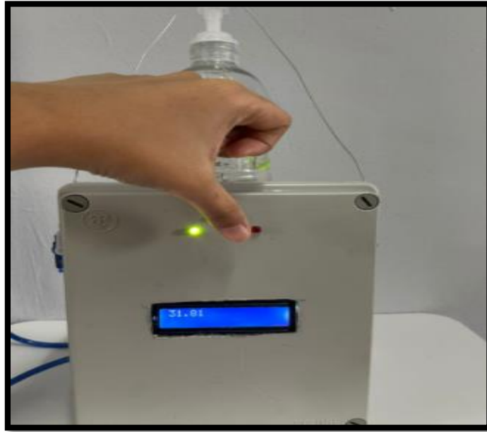
Figure 4.7: Temperature <37.5^{\circ}\text{C} and LED Green Turn ON
