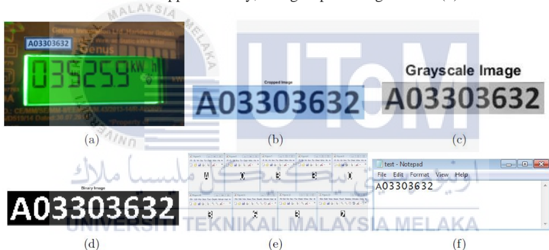
Figure 2.15 Step in Text Recognition
