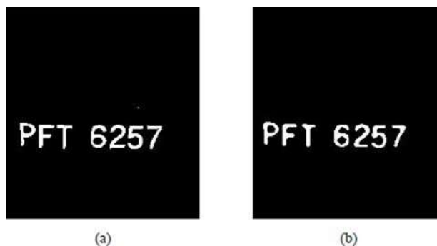
Figure 2.29 (a) Threshold Image. (b) Median Filtering Image
