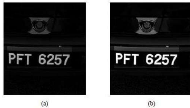
Figure 2.28 (a) Top hat filtering. (b) Contrast correction
