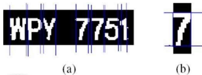
Figure 2.33 (a) Vertical segmentation (b) Horizontal segmentation
