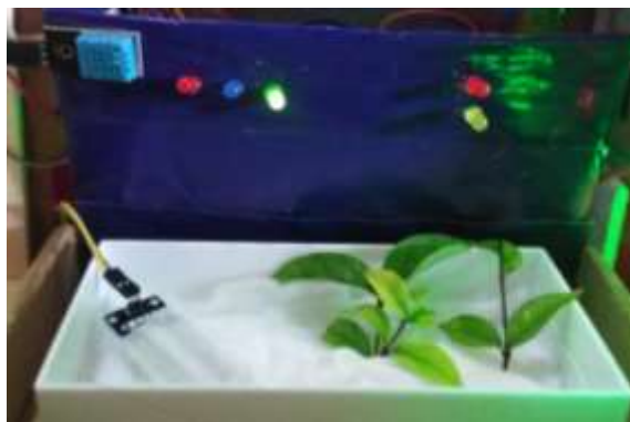
Figure 4.25 The Green LED will light up when the soil is perfect for plant.
