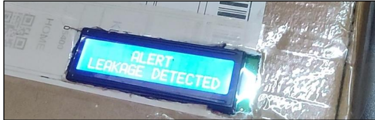
Figure 4.2 Leakage Detected and LCD Screen Show the Alert
