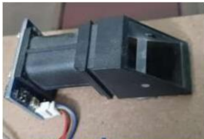
Figure 2.2: Example of Fingerprint Module
