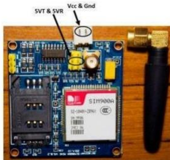
Figure 2.4 : Example of GSM SIM900A module
