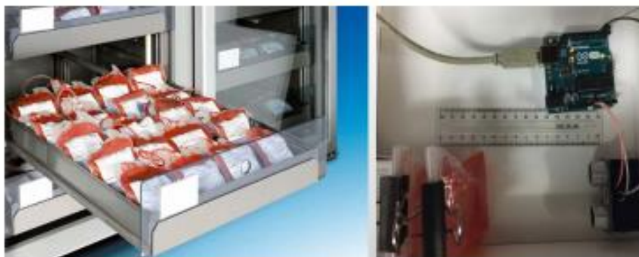
Figure 2.14 IoT based ultrasonic sensor in blood bank refrigerators.
