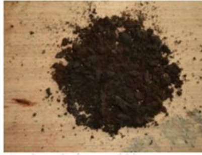
Figure 2.27: Steel wool after scrubbing the raw biogas
