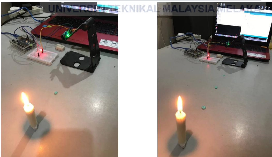
Figure 4.6: Flame sensor detect fire at 0.02 and 0.04 meter
