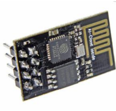
Figure 2.46: ESP8266-01 WiFi Module
