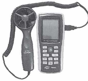
Figure 3.7: Air flow anemometer
