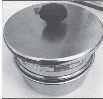
Figure 3. 6: Size of 75 \mu m of stainless-steel sifter
