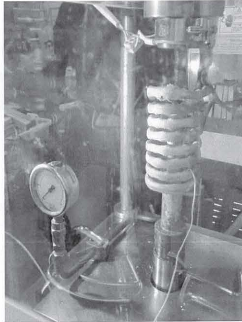
Figure 3.4: Induction coil in Thixoforming Machine
