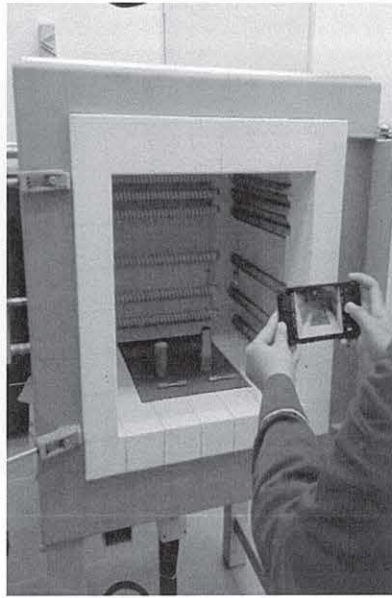
Figure 3. 7: Furnace for T6 Heat Treatment
