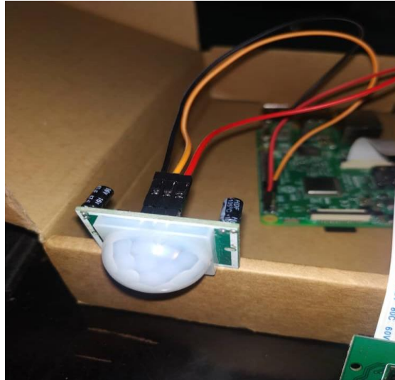
Figure 6-2 Successful wired PIR sensor
