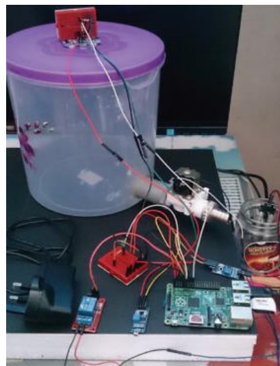
Figure 2.9: Prototype of Smart Home Garden Irrigation System
