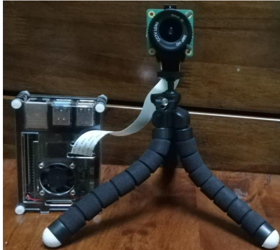
Figure 5.3.1 Prototype of Smart CCTV camera with face recognition.
