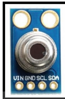
Figure 4.9 Infrared Thermometer MLX-90614
