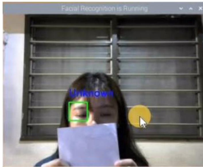
Figure 6.6: Face captured not matched with the dataset (face not recognized)
