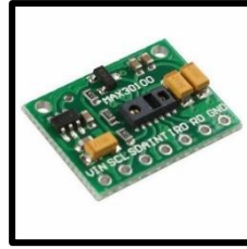
Figure 2.2: Components of MAX30100 Sensor (Pixel Electric)
