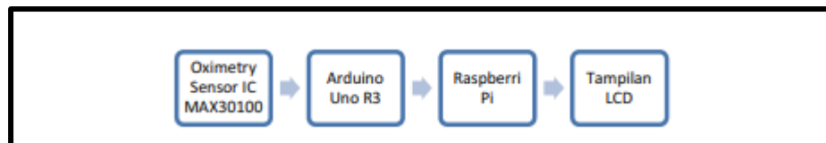
Figure 2.7: Concept Design of Design Low-Cost Oximetry Based on Raspberry Pi (Bakhri, S., Rosiana, E., & Saputra, R. C., 2020)
