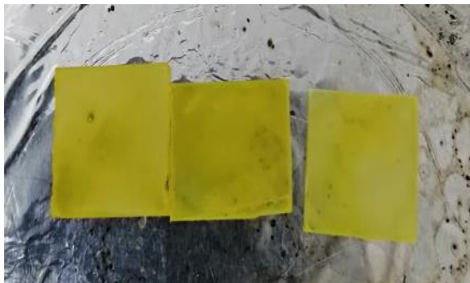
Figure 3.27 Yellow form from PbI 2 deposition
