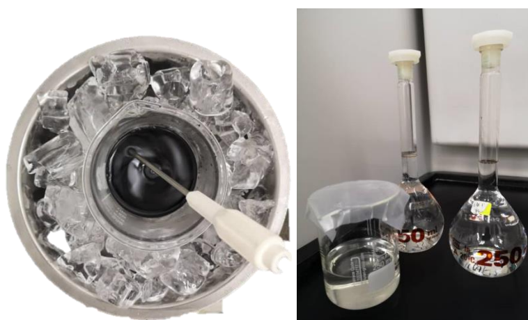
Figure 3.21 Ice bath and measured sulfanilic acid, HCl, and distilled water.
