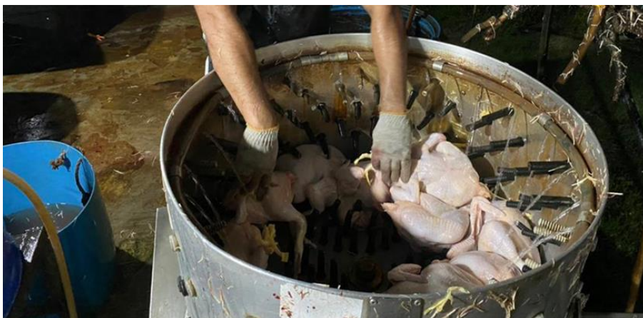
Figure 4.9: The plucking machine used in the industry
