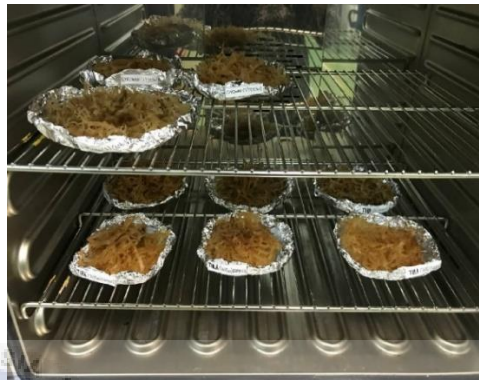
Figure 3.7: The drying process on seaweed (10h, 60°C)
