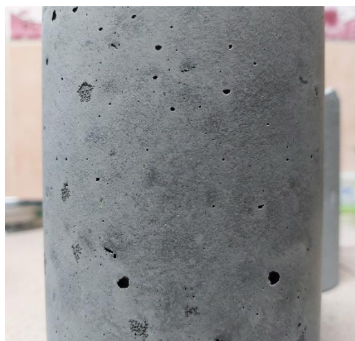
Figure 4.4: Concrete with Recycled Glass Fiber
