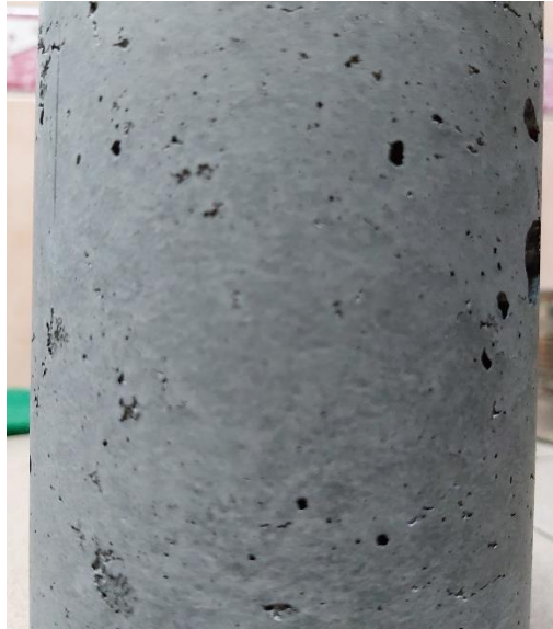
Figure 4.5: Concrete with Recycled Carbon Fiber
