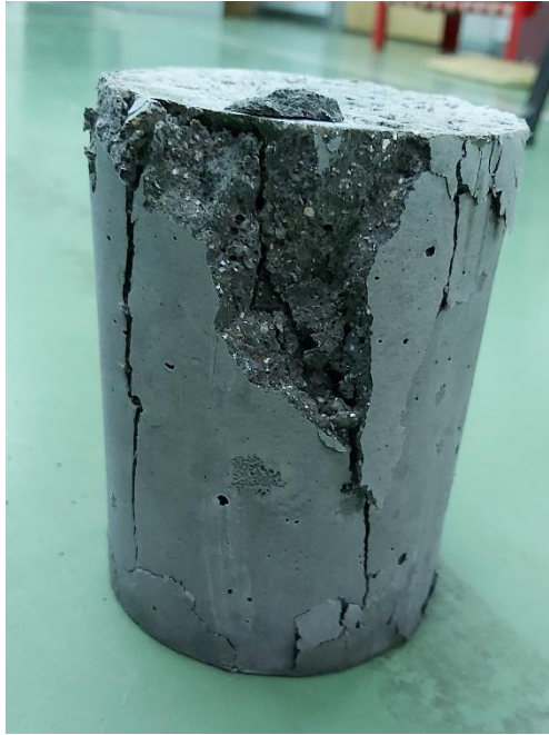
Figure 4.11: Fracture of Concrete with Recycled Glass Fiber
