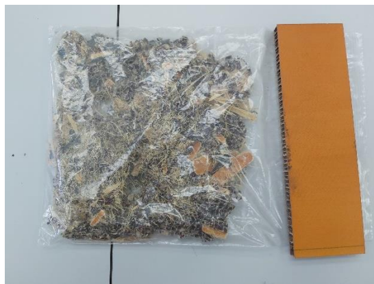
Figure 3.6: Recycled glass fiber after shredding process
