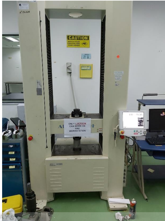
Figure 3,9: Compressive Testing Machine
