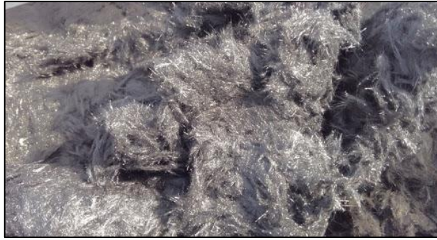
Figure 2.5 Recycled fibrous product of CFRP (Milberg, 2018)
