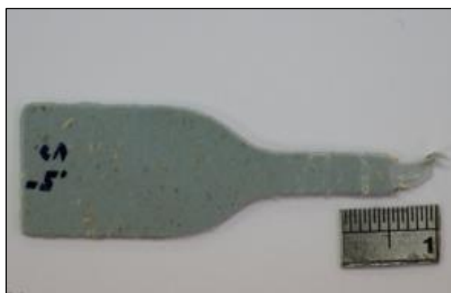
Figure 2.13 Tensile fracture sample (Khanam et al. , 2015)
