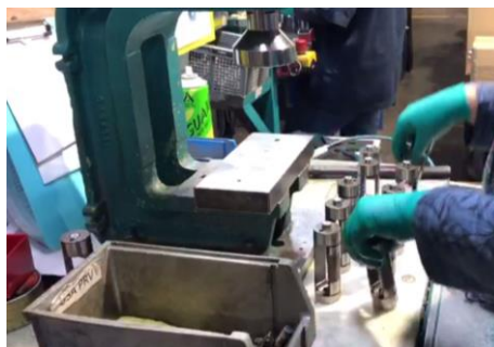
Figure 4.7: The operator immediately invert the piston each time after pressing the PLV inside the piston (after 2 pieces)
